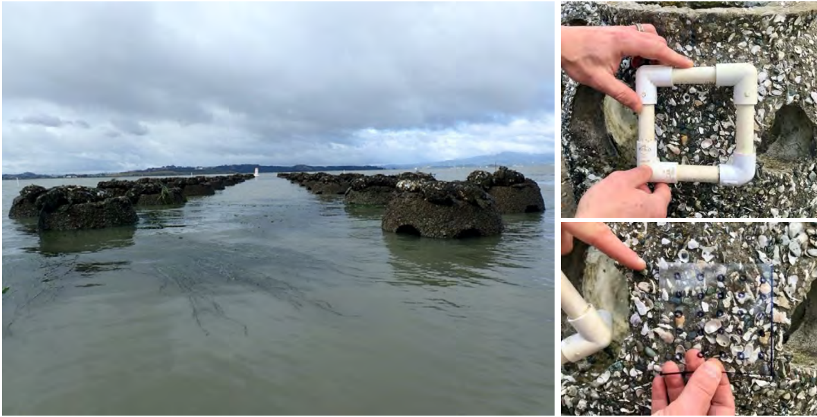
Figure 5. Left: An array of oyster/habitat reefs in Treatment 1, showing reef balls topped with bags of Pacific oyster shell. Eelgrass in the foreground was present prior to the project installation. Right: Monitoring with a quadrat (top) and acetate sheet (bottom).
